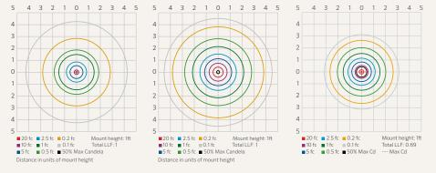
Beam angle is calculated using LM-79 method for SSL Luminaires: "Beam angle is defined as two times the vertical angle at which the intensity is 50% of the maximum." LISTED
