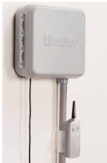
Roam Remote Control Kit The Hunter Roam Remote Control Kit saves time during installation and routine system maintenance. The receiver (left) plugs into the Controller Connection Kit and the transmitter (above) activates the sprinklers within a 1000' range. The user can manually run any zone without resetting the controller.
