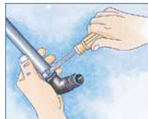
Poly Pipe: 2. Tighten clamp around pipe and fitting.
