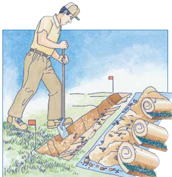
First lay down tarps and remove sod, then dig trenches 10" to 12" deep for the main line. Trench 6" to 8" for lateral lines.
