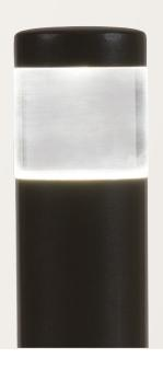
Designed for mid-sized landscapes, the PM is engineered without compromise in the spirit of a large contemporary commercial bollard. Precisely milled from 6061 T-6 alloy, this model looks and performs like no other. Computer-designed parabolic reflector, diffuser cone and optics work together to produce long projection beam spread with no glare.
